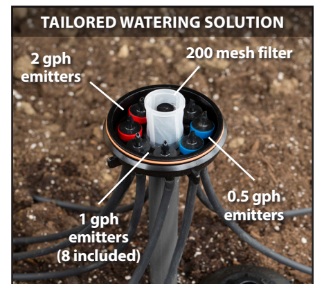
Each port can be configured on the Xeri-Bird™ by installing flow controlled emitters. Above shows a combination of 0.5, 1.0, and 2.0 gph Xeri-Bug emitters. Below is a list of available emitters.
